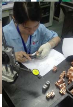
电极卡尺检测
